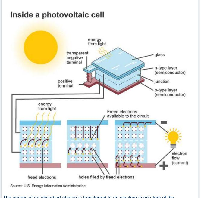
The energy of an absorbed photon is transferred to an electron in an atom of the semiconductor device. This energy allows the electron to escape from its normal position associated with a single atom in the semiconductor device to become part of the current in an electrical circuit.
